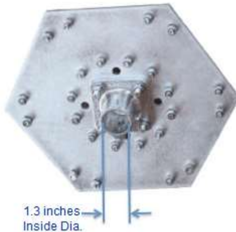
Base plate bottom with flange that slips onto the mast.
