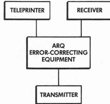
*A minimum equipment configuration for direct-printing may have this form.*
