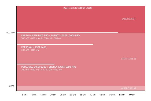
Distance measured from laser diode, laser tip, optical fibre, or collector lens. Power measurements are made using Molectron POWER MAX 500AD Laser Power Meter.
