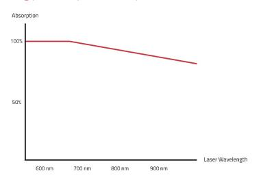
Measurements carried out using Molectron POWER MAX 500AD Laser Power Meter shows that the laser energy from 660 nm absorbs 100% and from 808 nm the laser energy absorbs 96 % by direct illumination on the green special glasses.
