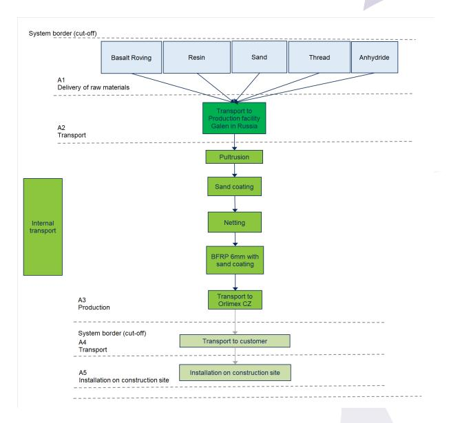
Figure: LCA process diagram according to EN 15804 (7.2.1)
