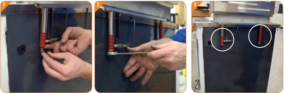
Step 4 : Mount springs on both sides and tighten screws
