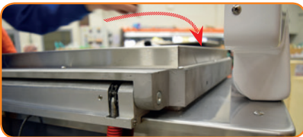
Step 6: Close the gridframe onto the machine
