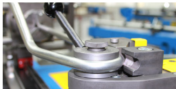
Fast and easy bending of pipe shapes up to \varnothing 20 mm.
