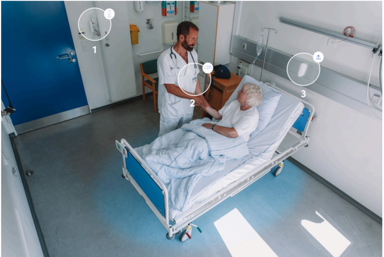
Fig 1. The Sani nudge hygiene system in a hospital patient room. 1. A Sensor on a dispenser registering the number of alcohol-based hand rubbing events; 2. An anonymous sensor on the name badge of each healthcare worker. The sensor is coded according to staff profession. 3. The patient zone (illustrated with blue) created by the sensor near the head of the patient bed. Data captured by the sensors are sent to a secure cloud-based server and stored at the device level. The two persons in the figure are volunteers and not part of the study.
