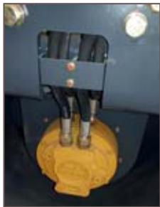
Lubrication point on each cylinder and Poclair drive motors
