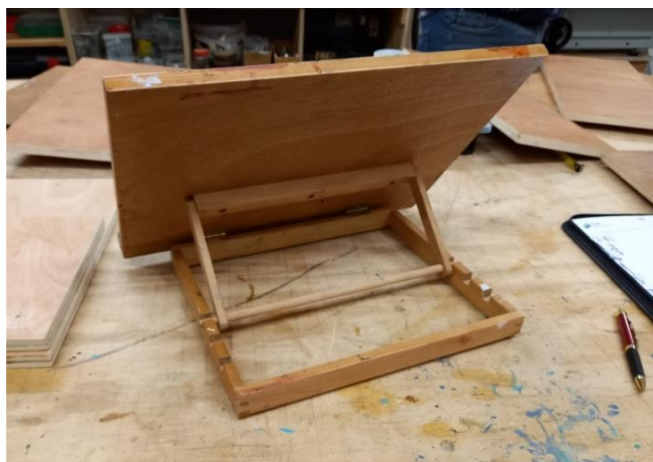
This is the model he provided for the design of the easels. In the background are the blanks ready for assembly
