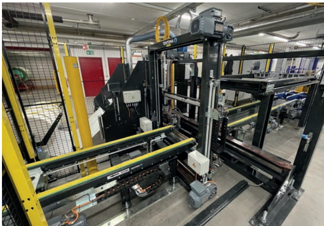
The RoRo StretchPack® packaging machine, installed by Tentoma A/S, is part of a new, fully automated production line at Getzner Textil AG's production facilities in Bludenz, Austria.
