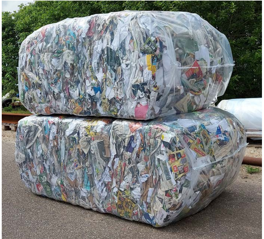
Waste bales packed in a single-layer tubular film by RoRo StretchPack®.
