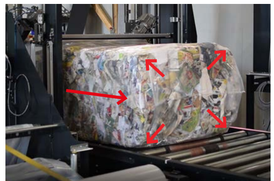
The RoRo StretchPack® packaging process
