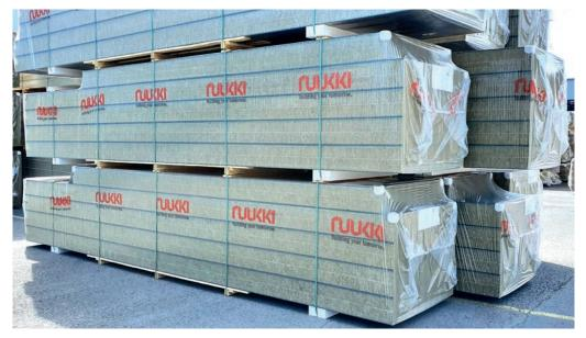
The new packaging is smooth and tight, and with the printable film, the packed sandwich panels are now branded nicely with the Ruukki logo.
