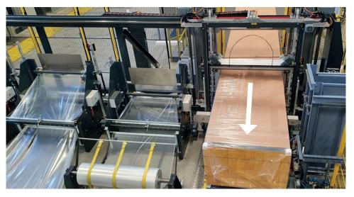
A stack of Ruukki sandwich panels is packed and sealed in one operation with the RoRo StretchPack® machine. Ruukki does not need an extra process to cover the panel ends anymore.
