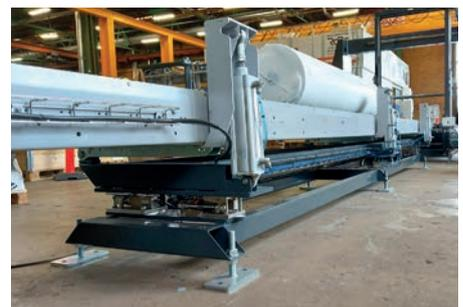
Tilt conveyor with load cells
