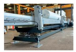
Tilt conveyor with load cells
