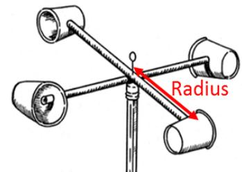
$$\begin{array}{ccccccc} \text{Angular velocity} & & \text{Conversion} & & \text{Anemometer} & = & \text{Linear velocity} \\ \text{(rotations/second)} & * & \text{from (rev/s) to} & * & \text{radius (meters)} & = & \text{(meters/second)} \\ & & \text{(rad/s)} & & & & \\ \hline & * & \underline{2 * \pi} & * & \hline & = & \hline \end{array}$$
