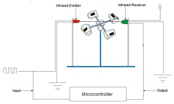
Fig 1: Setup of Indigenous Infrared Wind speed Sensor
