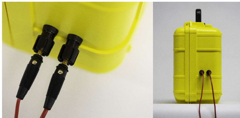
Figure 7. sTEM banana plugs. Connect Tx coil in any order.
