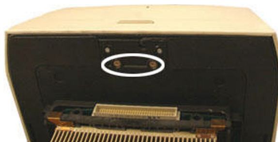
Figure 121. Remove these screws to unlock the optical module.
