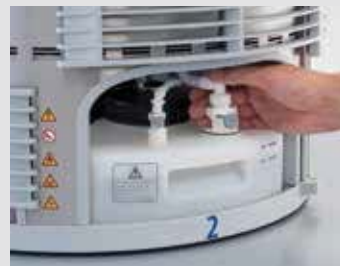
Connecting media containers
