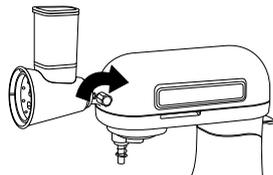
Tighten the attachment fixing screw
