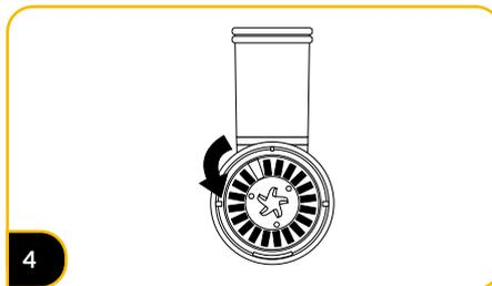
**4** Carefully put your hand inside the blade, lift it slightly upwards, shake it gently and slide it out by turning the blade counter-clockwise.
