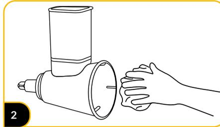
2 Wipe off any water or food residue with a cloth. **Note: the knives are extremely sharp, it is recommended to use protective gloves.**
