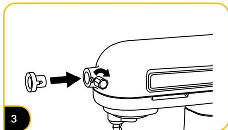
**3** Place the cap of the attachment socket, then tighten the retaining screw.
