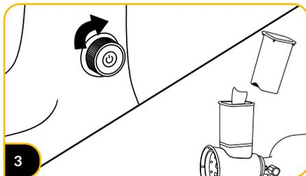
Run the device at the selected speed (recommended level: 4-6). Insert the pieces of food one at a time and push them slowly using the provided pusher.
