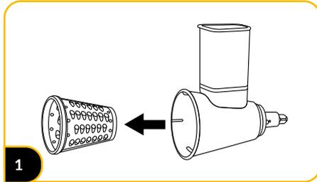
1 Remove the blade from the slicer. Wash all parts with soap and water.
