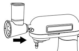
Insert the attachment into the mixer interface. To make sure the shaft is stuck in the interface slot, rotate the blade left or right as needed. When the fit is correct, the pin in the accessory housing will fit into the groove on the edge of the bushing.
