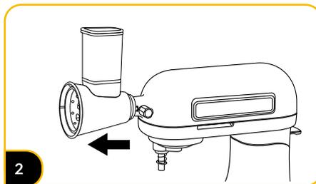
**2** Loosen the screw that secures the attachment, and then slide the attachment out of the slot.
