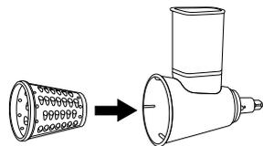
Insert the selected blade into the attachment body
