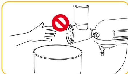
Note: If excess grated ingredients get stuck in the grater, do not try to empty it with your fingers when the device is on. Turn off the device and remove the attachment before removing the excess.
