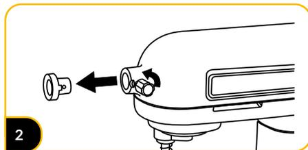
2 Loosen the attachment screw and remove the socket cap.
