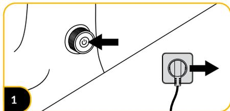
1 Turn off the food processor and disconnect it from the power supply.
