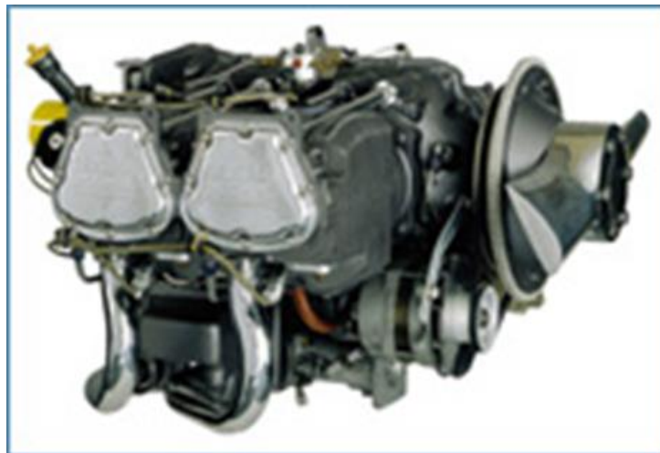
Kolvmotor Ly5 (Lycoming IO-360-A1B6)
