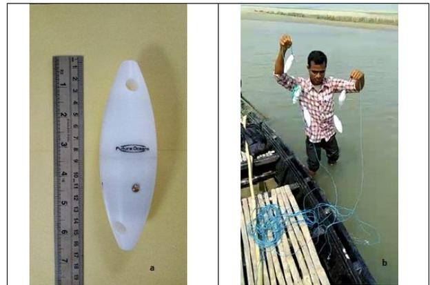
Fig. 2 a. Pinger, b. deploying in Freshwater
