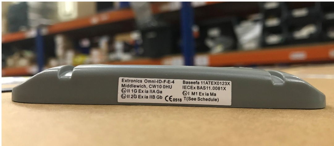
Figure 8: Close up view of iTAG500 hazardous area markings
