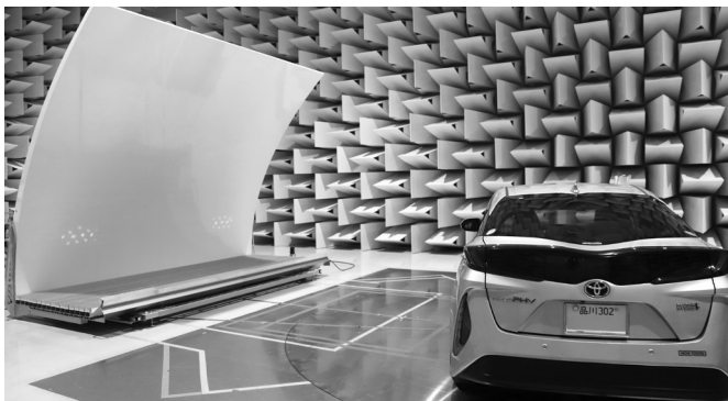
(17) RanLOS test system in an EMC chamber
