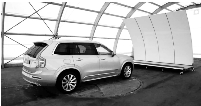
(18) RanLOS test system in a weather-protected open-area test site during SIVERT - a FFI-Vinnova project
