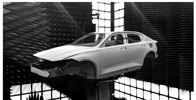
(19) RanLOS test setup placed in a test tent compared with an advanced test facility in Denmark. These measurements were done during SIVERT - a FFI-Vinnova project
