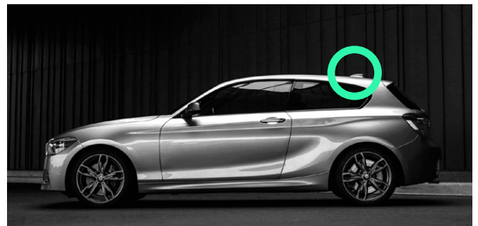
(1) Roof-mounted antenna with a position at the rear of the roof
