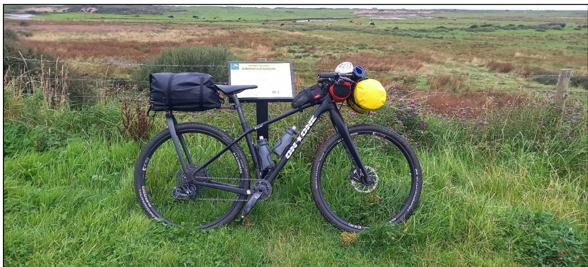
Bike set-up: Whippet XC (carbon-fibre) 29" wheels, Tailfin (rear) and Aeroe Frame (front)
