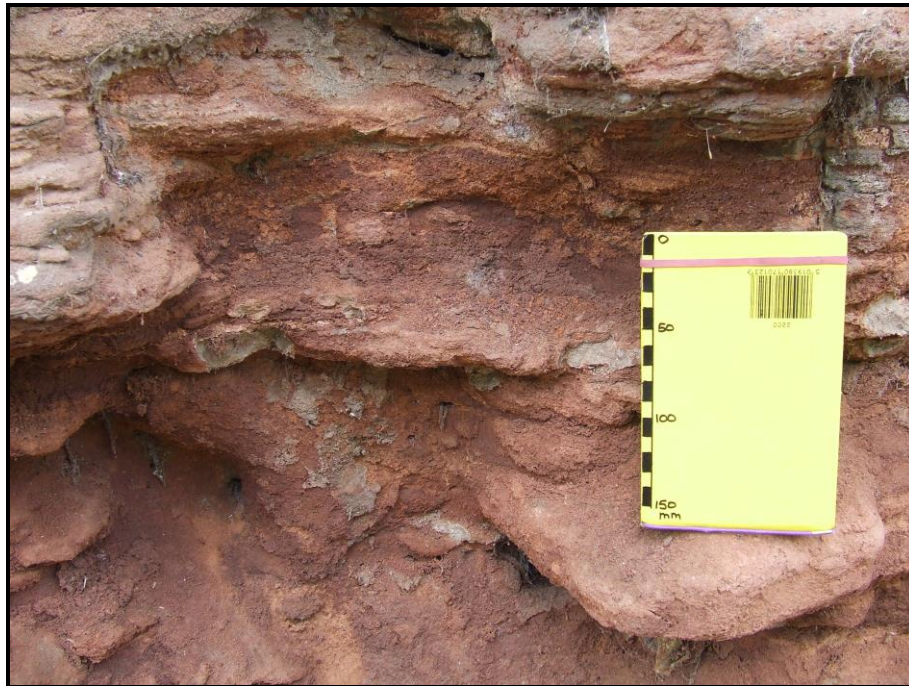
Figure 7. Sandstone exposed in a roadside cutting at NGR ST 5960 6056. Weathering and erosion of the material is apparent.
