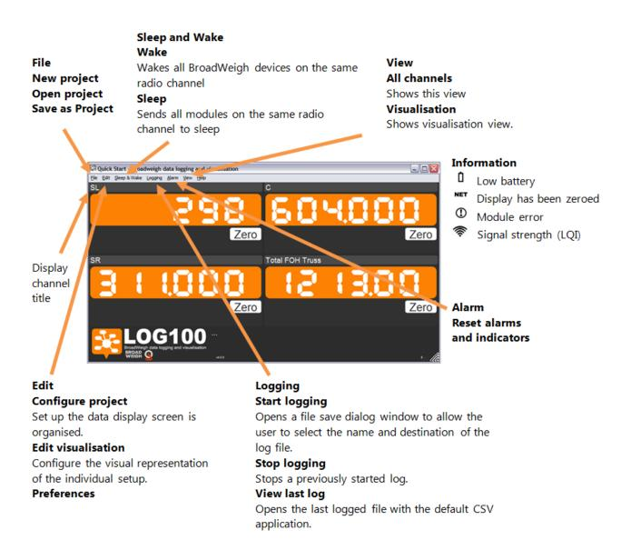
A window similar to the one above will appear (four display channels are shown). This is the all channels display window. Each display channel does not necessarily need to display data from a single BroadWeigh shackle; they can be set up to show mathematical calculations involving as many shackles as required.
