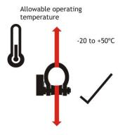
The working load limit (WLL) of BroadWeigh shackles assumes the absence of exceptionally hazardous conditions. These include offshore activities and lifting of potentially dangerous loads such as molten metals. With every use the degree of hazard should be assessed by a competent person and the safe working load (SWL) reduced accordingly from the working load limit.
