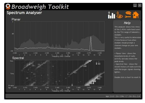
The previous charts show the traffic from a Wi-Fi network and it can be seen to be operating over channels 12 to 16. It would be best (though not essential) to avoid using these channels. One of the useful features of Group Keys is that an entire group can move radio channel all at the same time.
