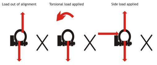
If using the shackle as part of a bridle, remember that the load in legs of the bridle will increase with the angle. If the Broadweigh shackle pin is not connected to that part of the leg then it will not register this increase.
