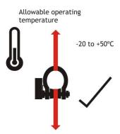
The working load limit (WLL) of Broadweigh shackles assumes the absence of exceptionally hazardous conditions. These include offshore activities, lifting of persons and lifting of potentially dangerous loads such as molten metals. In such cases the degree of hazard should be assessed by a competent person and the safe working load (SWL) reduced accordingly from the working load limit.
