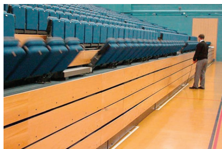
Semi-Automatic - chairs are automatically folded down as the platforms close, and picked up in groups of up to 14 after the platforms have been opened.
