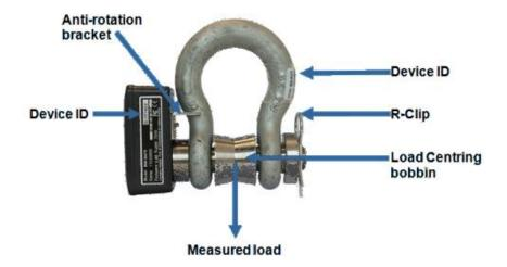
Any out of alignment, side or twist loading will affect the readings given as well as load the shackle in a way that it was not designed for.
