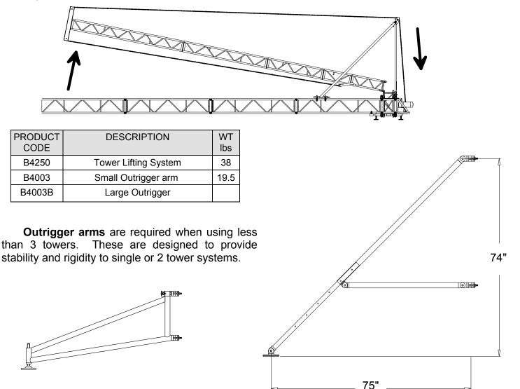
The ground support tower system can be used outside but must be suitably anchored from the top of each tower sleeve block to the ground via a guy wire to a suitable ground anchor. We recommend that the bases are sat on top of a 3' square piece of 3/4" plywood. Should a cover be required please refer to James Thomas Engineering for an approved design to suit your requirements.
