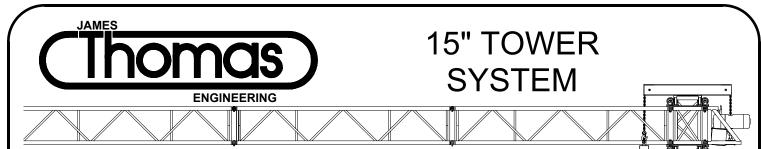
The 15" square ground support tower is a system manufactured for the purpose of providing a lifting medium for a variety of Thomas trusses from, 20.5" x 20.5", Heavy duty, Supertruss, and Pre-rig truss through to Roof systems.
