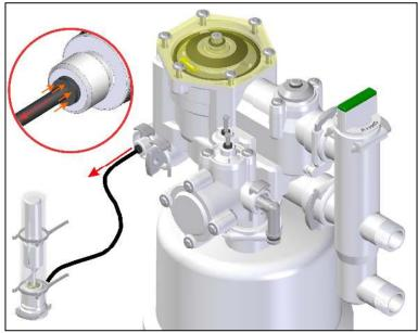
2. Connect one end of a piece of tubing Ø4 mm to the quick-connect fitting on the control valve; push it in as far as possible.
