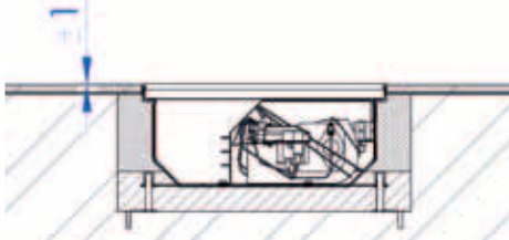
FIG. 22: A correctly installed convector has a standard frame aligned with the floor finish with a tolerance of ± 1 mm.
