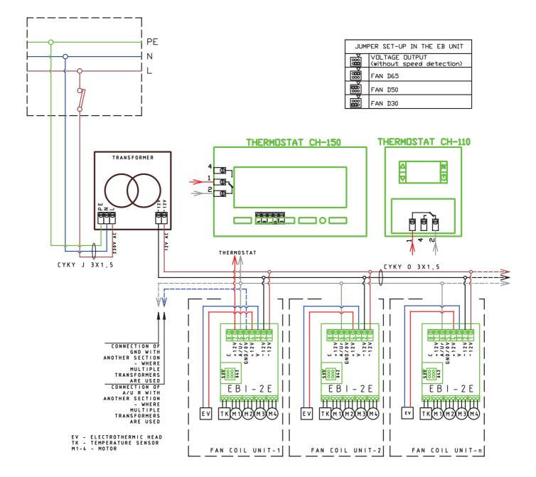
When connecting more than five convectors to one transformer it is necessary to connect the thermostat to the convector which in the branch that is closest to the transformer.
