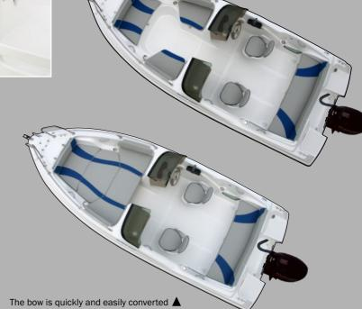
The bow is quickly and easily converted **\( \)** into a large bed for sunbathing and rest (optional equipment).
