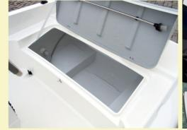
The ergonomically designed and robust console makes the journey comfortable for the driver by providing protection from the wind. At the same time, adequate space for the boat's instruments is provided, while the locker acts as storage space and provides easy access to the console's internals. **V**
