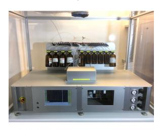
OligoMaker 768 and OligoMaker 1536 (screen) synthesizes 2 x 364 or 4 x 364 primere over night in one run
