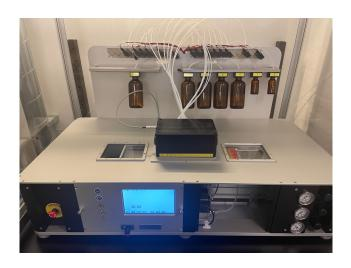
**OligoMaker X192/6** synthesizes 192 oligos (20-mer) in 3-4 hours. Reaction Plates 2 x 96 plate or columns (titre plate format)
