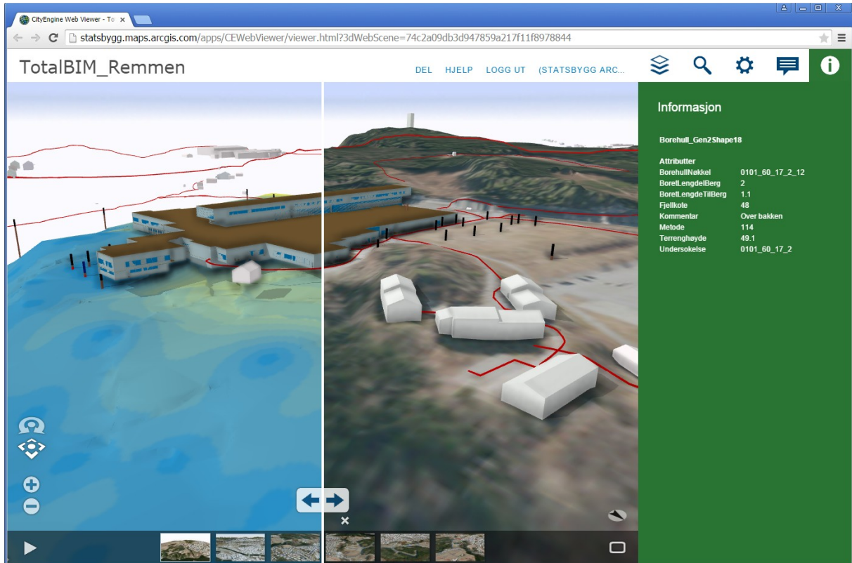
Figure 24: The College of Østfold campus in Halden in 3D; a GIS and BIM mixed model.
