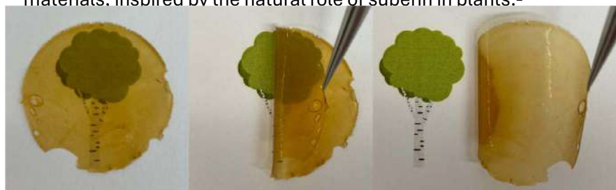
Figure 1. Sequence of picture showing the flexibility of the suberin-reconstructed film.
