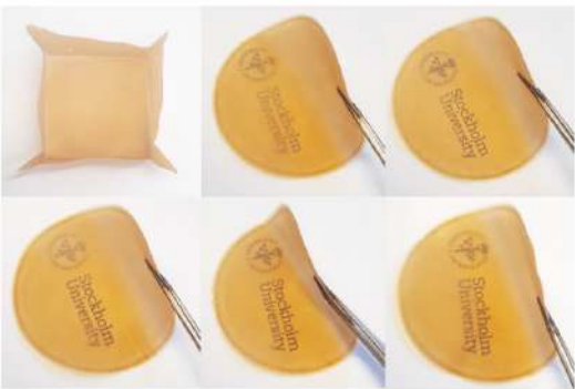
Foldability of L-MFC film and translucency at varying lignin content.
