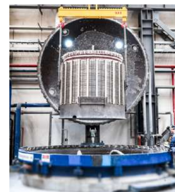
Stator lifted from pressure vessel
