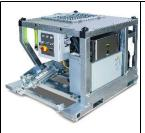
Underground conditions in tunnels and mines can be extremely demanding. The machine has been designed for maximum protection. The pump easily manages soil consolidation works injection grout work as well as void filling and back filling applications.
