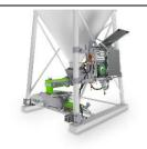
The MAI®HICOMP is the perfect big silo mixing pump for large volumes, with an adjustable pumping capacity of 100 to 170 l/min (with a nominal mortar hose diameter of 50mm and distance of approx. 100 m) and a grain size of up to 6 mm or even up to 8mm (although this may lead to increased wear) for a silo flange diameter of 350 mm.
