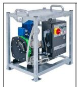
The MAI®DOS is a universally applicable dosing unit for liquid additives in a foam concrete production system. Dose additives at between 5 l/h and 160 l/h at up to maximum 12bar pressure. It is suitable for use with the MAI®HICOMP, MAI®MULTIMIX and MAI®440GE mixing pumps.
