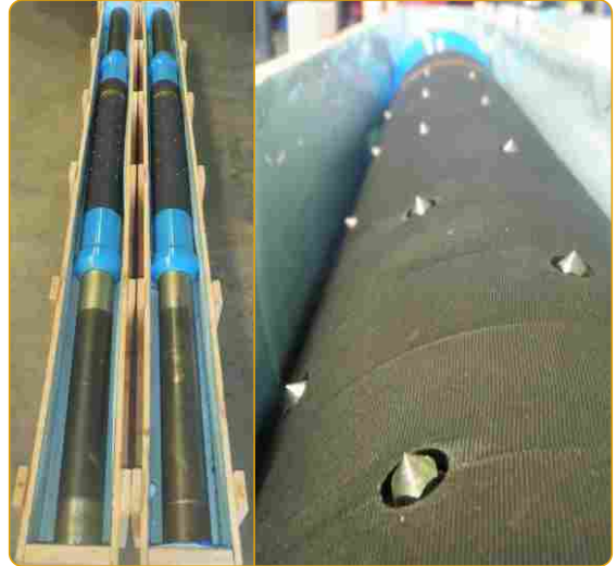
Special purpose inflatable packers deployed as part of a subglacial geological drilling operation performed for an Antarctic research project. This is another IPI supplied project funded by the United States Government. IPI has clients on every continent, including those operating in Antarctica's extreme conditions.
