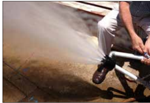
9x8 Cluster Nozzle being tested on surface
