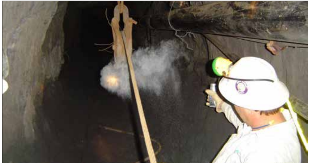
Airflow velocities being tested underground
