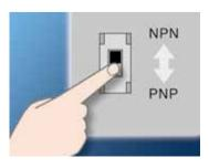
iE5 provides both PNP and NPN minor signal powers so that no matter what signal type the external controller adopts, +24V power can be applied.
