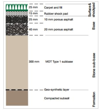
Typical build-up for an artificial surfacing system
