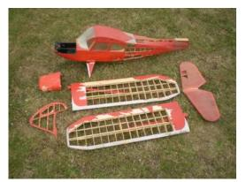
When I first set eyes on the beast I was surprised to see that structurally it was virtually undamaged apart from the red tissue covering. However, as I intended to install radio control, several modifications were required. Firstly, for free-flight, the tail surfaces and wing panels were
