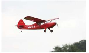
held on by thin rubber bands so that they would "knock off" in the event of a crash. Therefore, after incorporating elevators and a decent size rudder, I glued the tail surfaces in place and beefed up the wing mounting arrangements and struts. I also beefed up the undercarriage to allow for the extra weight of R/C gear etc. The receiver and servos were then located under a hatch aft of the wing. Fitting
