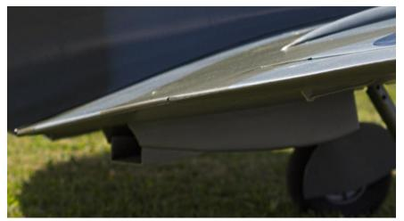
Yet another radio channel is used for opening the radiator ducts.
