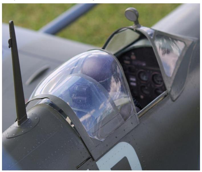
The canopy uses up a channel on the radio because it slides back under servo control.
