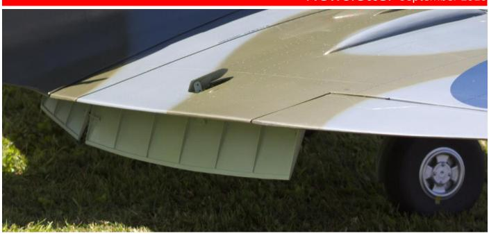
The flaps include the scale popup doors on the top side of the wing to allow clearance for the actuator horn. It also gave the pilot a visual indication of the flap position.
