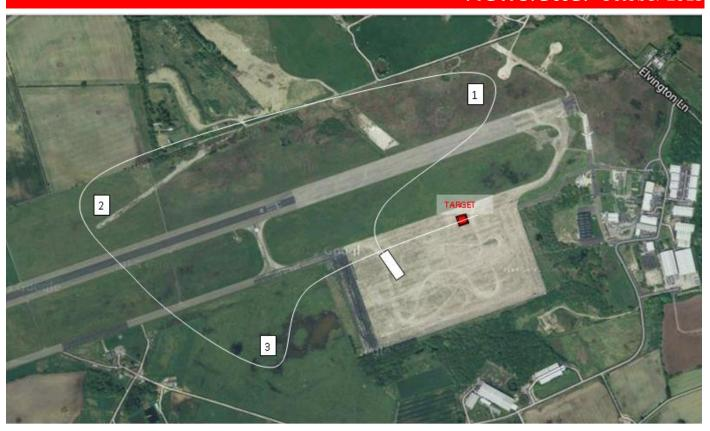
Take-off was conducted within a designated take-off and landing box, into wind. After take-off the system had to maintain steady controlled flight at a height of 100 ft.
