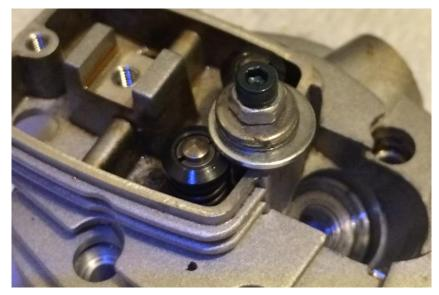
(taken after I got the valve assembled). As the screw was one of the actual rocker cover screws, it was a bit long for this job, hence the nut and other washers acting as spacers.
