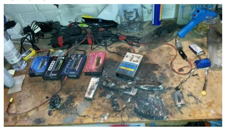
It all started when the blue and silver charger near the centre of the picture was being used to charge the Turnigy Orange TX directly in front of the charger. OK, I hear you saying "what Orange TX?" Well, it's that rectangular mess that is actually just the PCB and a few miscellaneous components that weren't completely annihilated by the fire.
