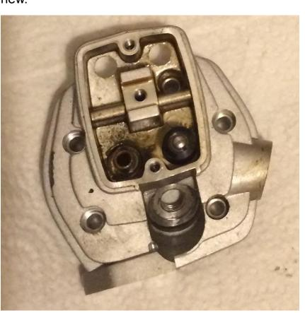
I expect that most are familiar with the process of removing valves but if like me you've never done it before, then what you have to do is support the valve from underneath (I just used a finger but wood is a good alternative), then compress the valve spring by pressing down on the retainer cap.
